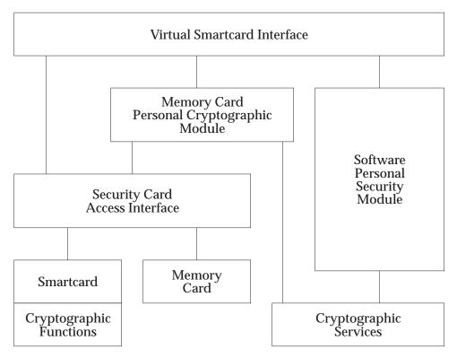
Figure 4-1 Hardware Security Devices
