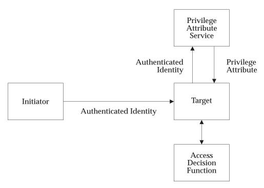
Figure 3-14 Pull Model of Access Control
