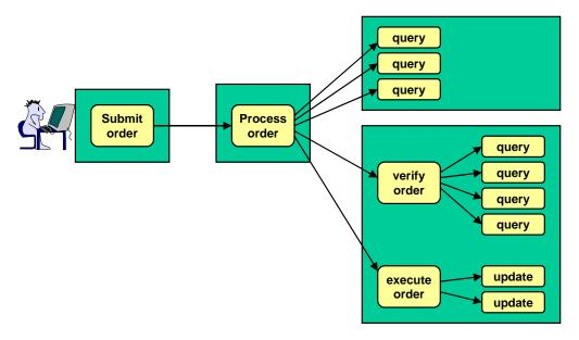
Figure 9: An Example of a Distributed Transaction
