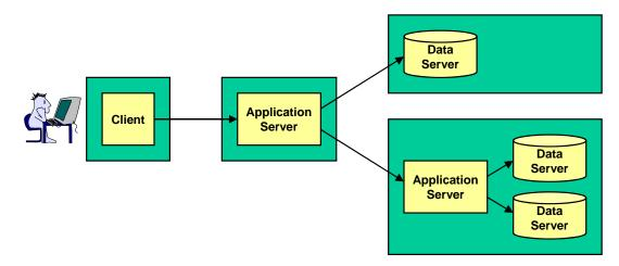
Figure 8: A Common Distributed Application Architecture
