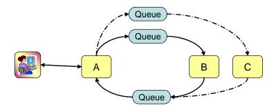
Figure 13: Request/Response with Parallel Asynchronous Flows
