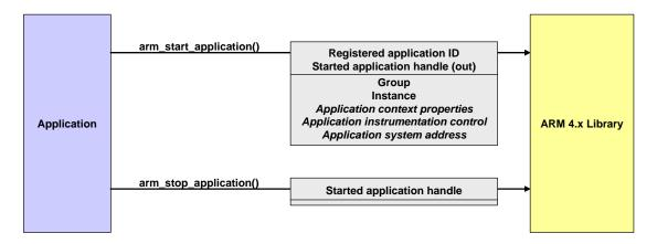
Figure 21: API Functions for Application Starts and Stops
