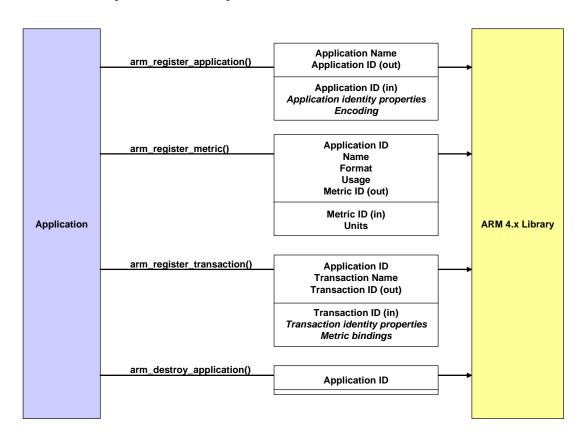
Figure 20: API Functions to Register Metadata
