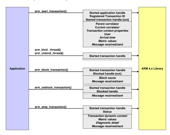
Figure 22: Most Frequently Used API Functions to Measure Transactions
