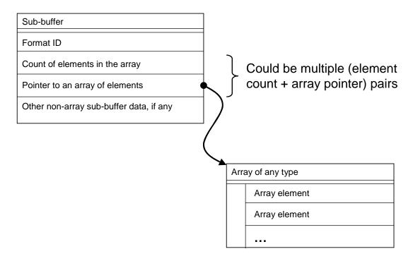
Figure 25: Format of Sub-Buffer that Contains One or More Arrays of Data
