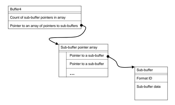
Figure 19: Structure of Optional Buffer and Sub-Buffers
