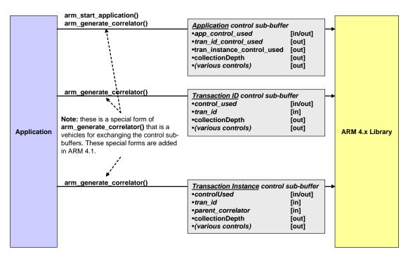
Figure 23: Instrumentation Control APIs
