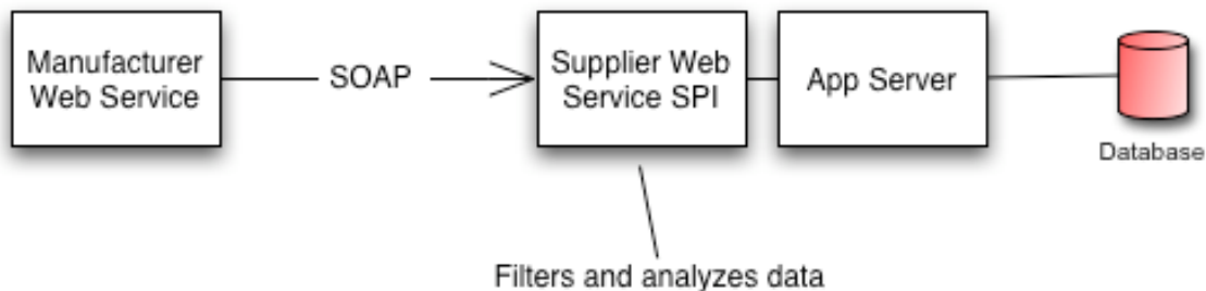
Figure 3: Security Pipeline Interface provides data integrity and logging
